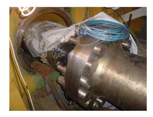
Here Boltight tools are about to be employed to tighten M76 and M90 bolts on the propulsion shafting of large naval vessels.
